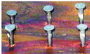
PT2000™ fastener after 1008 hours salt spray
