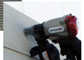
Fiber Cement Siding to Steel
