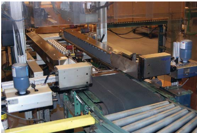
TWO-SIDED. Two ink-jet print heads are positioned on either side of the packaging line conveyor and are mounted to a box taper for easy changeover.
