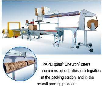
At a standard packing station system, the paper padding is located in a plastic tube at an ergonomic working height, ready to grab. The strip of padding is automatically divided into sections.
