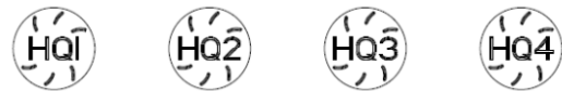
FIGURE 1. Head identification for HurriQuake® Nails, HQ1: 2-1/2x0.113 inch, HQ2: 2-1/2x0.131 inch, HQ3: 3x0.113 inch, and HQ4: 3x0.131 inch.
